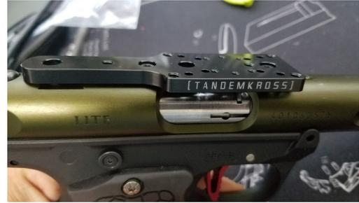
Use the two provided Torx size 10 socket head cap screws to attach the “Shadow” Mount to the receiver. Blue Loctite (medium strength) is recommended to keep the screws from loosening.
