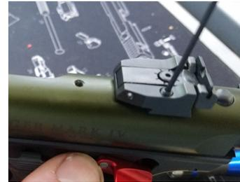
Remove rear sight assembly by pushing it out of dovetail slot from the left side of the firearm using a drift or sight pushing tool being careful not to damage the firearm. Sometimes the rear sight can be very tight in the dovetail and it may warrant a visit to your local gunsmith for removal.
